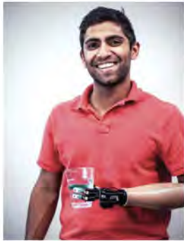
Smart prosthetic arm and hand with sense of touch
