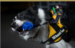
FIDO IS A WEARABLE COMPUTER TO HELP ASSISTANCE DOGS COMMUNICATE WITH THEIR HANDLERS
